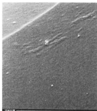
b). SEM photo: Clean fibre (2000X).
